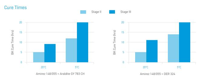
Faster curing can be achieved using solid epoxy resin such as BECKOPOX™ EP 2384w/57WA.
